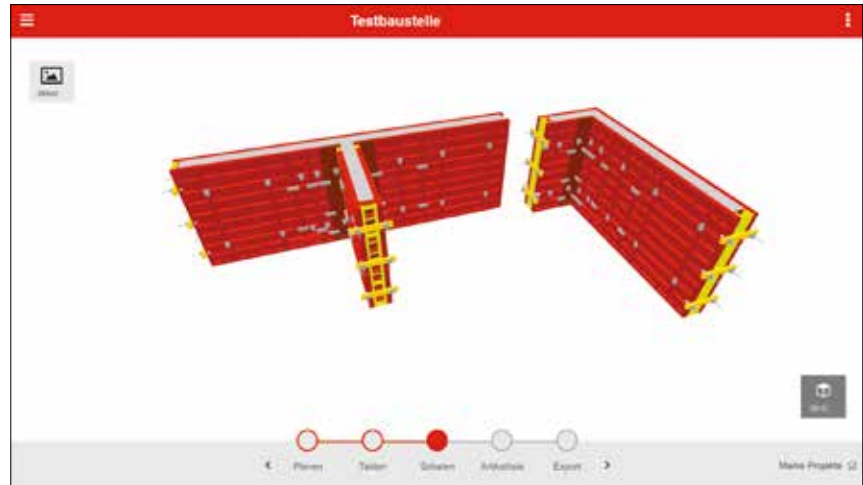
With the MAXIMO Planner, users can plan, cycle and shutter simple ground plans with the MAXIMO Panel Formwork System
